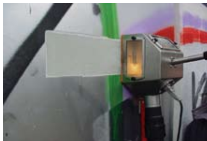
Foil friendly- smooth surfaces absorb the energy of grain blast. By covering lettering on a steel door with foil before blasting the remove layers of lacquer the wording will be undamaged. It is also ideal for removing paste from shop windows.
